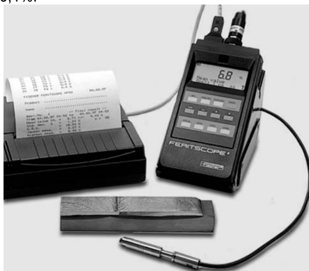
Fig. 19. The Fisher MP 30E-S Feritscope Sl. 19. Fisher MP 30E-S Feritscope
