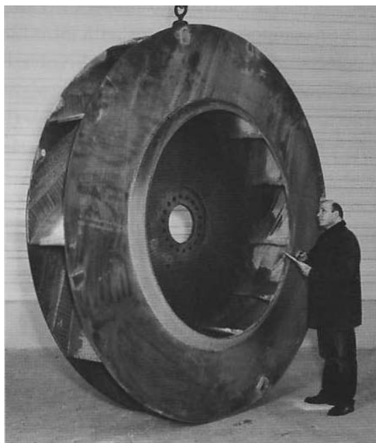
Fig.1. Application of separate wear plates on the structural material of a worn-out industrial ventilator (5).
