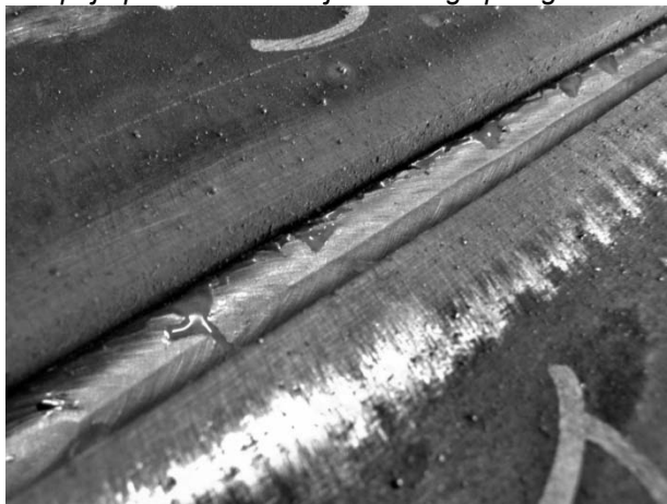
Figure 4. Joint 1 after the welding of the third fill weld. Slika 4. Spoj 1 posle zavarivanja trećeg zavara ispune
