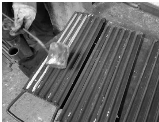
Picture number 3. The additional material are triangle bars (sides of the bar 6-10 mm) which are casted in a mould and immediately used in order not to come to the occurrence of surface oxidation of lead.
