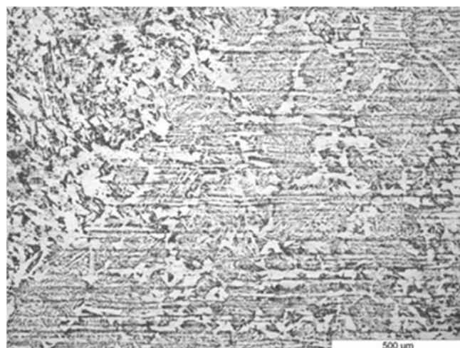
Figure 9 Fusion line and HAZ for welded sample S355J2+N, CGHAZ = 500 \mu m , HAZ = 1500 \mu m (visual delimitation), X500, nital
