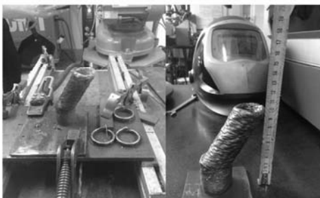
Figure 7. 3D model and final product welded by CMT and pulse combined process at welding current 59 A and welding speed 5 mm/s.
