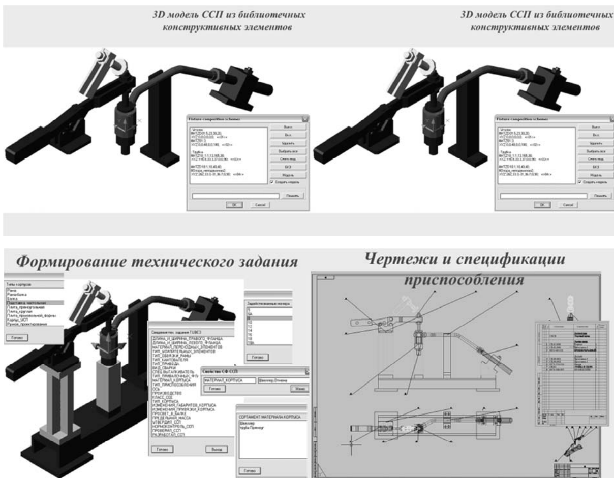
Figure 3. An example of the design of an assembly and welding device formed by the INSVAR software package Slika 3. Primer dizajna uređaja za montažu i zavarivanje formiranog softverskim paketom INSVARe
