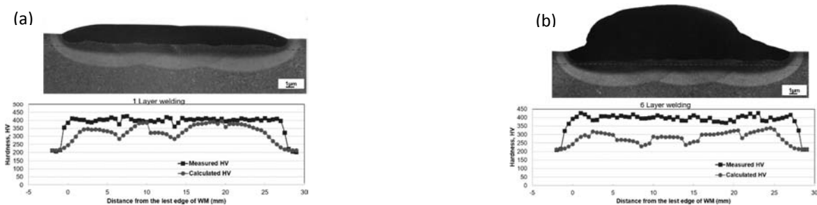
Fig. 17 Hardness comparison after 1Layer and 6Layer welding of A336 steel: (a) 1layer-3pass welding and (b) 6layer-21pass welding
