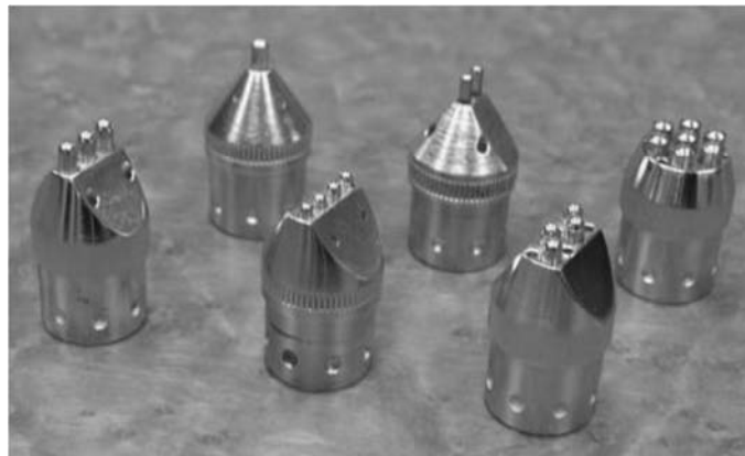
Figure 3. A set of interchangeable working heads for UIT/UP [1]
