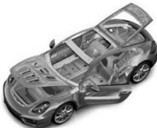
Figure 2. High strength aluminium alloys in a sport car-body [21]
