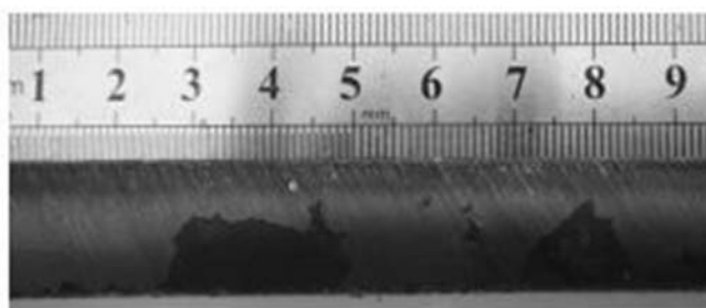
Figure 2. The surface morphology of water-air plasma cutting
