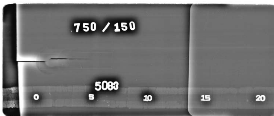
Figure 3. Radiograph of specimen 750/150, showing the presence of an inner channel
