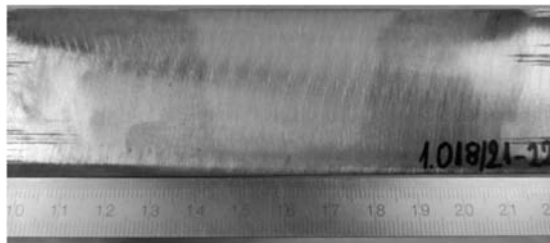
Slika 4. Makrosnimak uzorka navarivanog u normalizovanom stanju Figure 4. Macrostructure of the surface welded sample in the normalized condition
