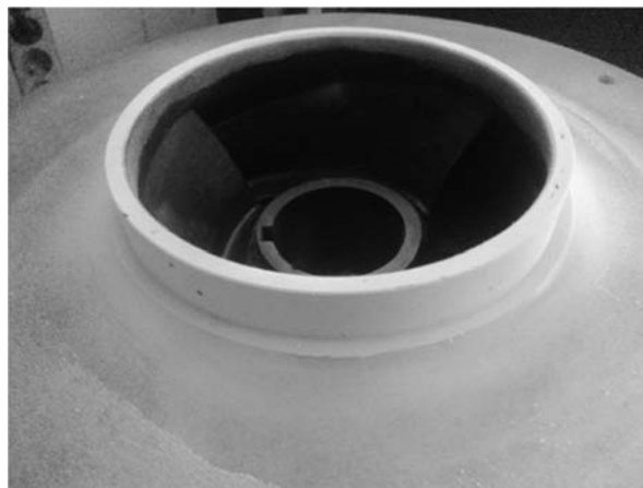
Slika 7. Kontrola penetrantima kvaliteta navara radnog kola Figure 7. Penetrant control of the quality of the working wheel welds
