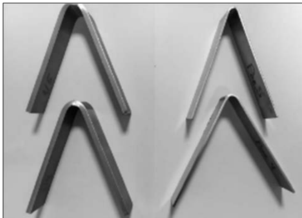
Figure 11. Bending tested samples
