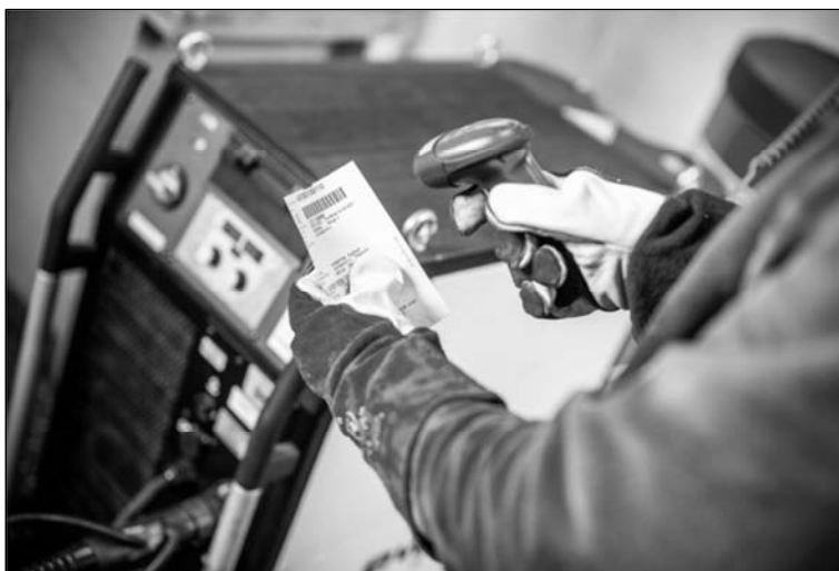
Figure 4. Welder scans the barcode on the component using a barcode scanner
