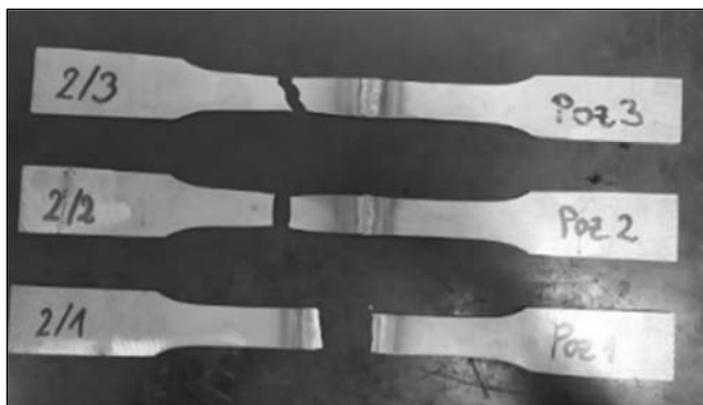
Figure 13. Tensile tested specimens from sample 2
