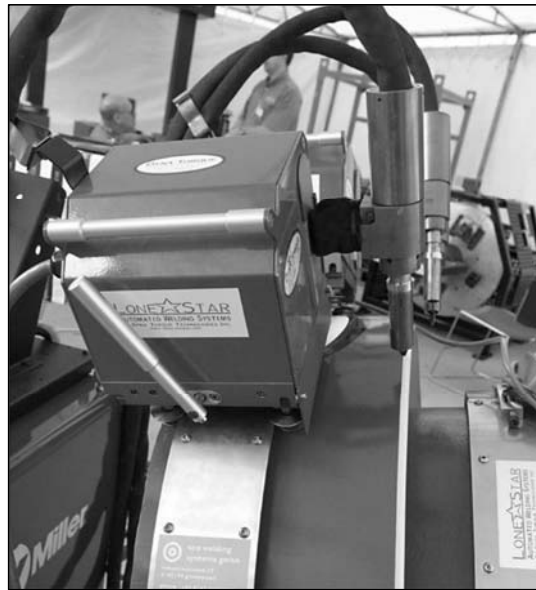
Figure 6. Automatic welding device with self-shielding wire
