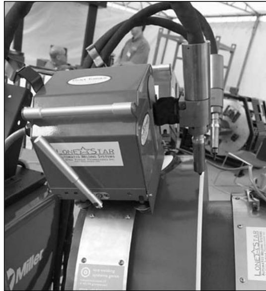
Figure 6. Automatic welding device with self-shielding wire
