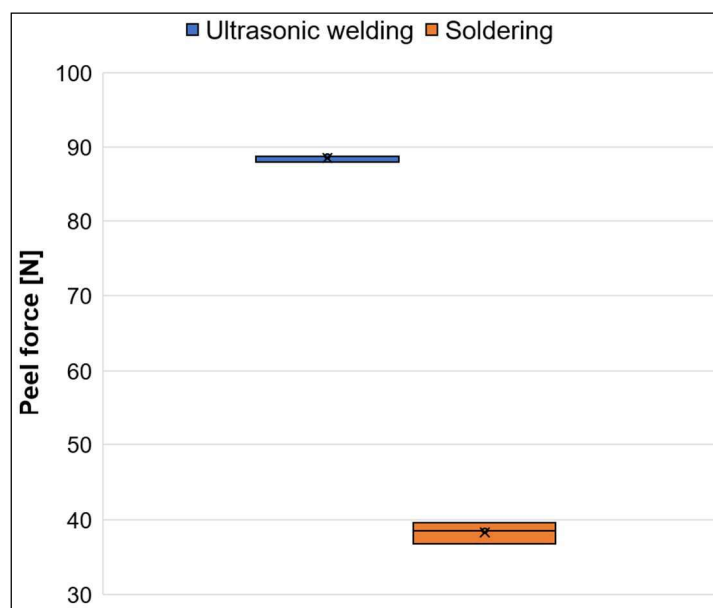
Figure 7. Comparison of peel force between UW joints (blue) and soldered joints (orange)
