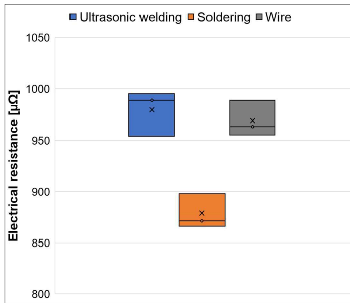
Figure 6. Comparison of electrical resistance between the UW joints (blue), soldered joints (orange), and wire (grey)
