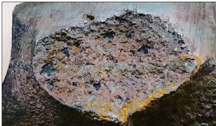
Figure 7: Example fracture surface of broken bucket tooth
