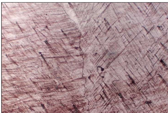
Figure 8: Work hardened manganese steel microstructure of the broken tooth
