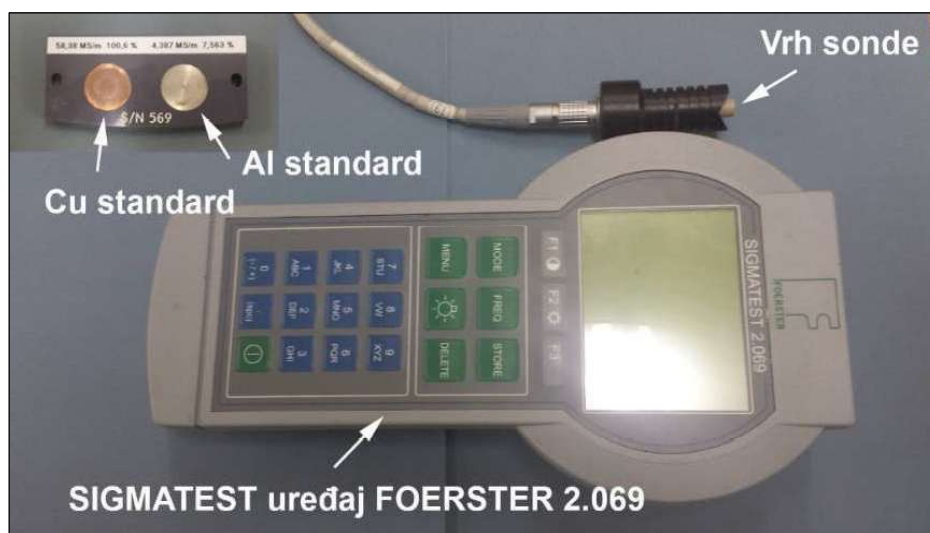
Slika 1. SIGMATEST uređaj sa mernom sondom ( \varnothing 8 mm) i kalibracionim standardima Figure 1. SIGMATEST device with measuring probe ( \varnothing 8 mm) and calibration standards
