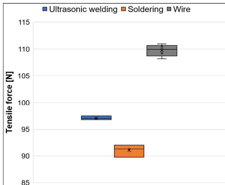
Figure 8. Comparison of tensile force between UW joints (blue), soldered joints (orange) and wire (grey)
