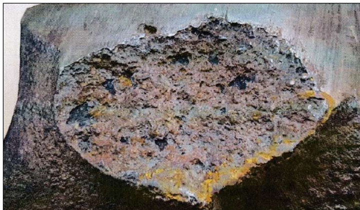
Figure 7: Example fracture surface of broken bucket tooth
